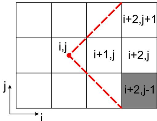
Fig. 5: Illustration of the transition block operation, we illustrate a 2D case analogous to the 3D case. In this example each visible block is visited to obtain the visible set of primitives that belongs to them. In this illustration we indicate that the visible face of block  $(i + 2, j - 1)$  is fully filled, so the next adjacent blocks are not directly added to the visitation queue due to it(they might be added due to another block).
