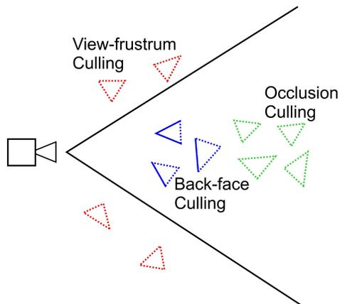
Fig. 1: Types of visibility culling techniques: view-frustum culling (in red), back-face culling (in blue), and occlusion culling (in green).
