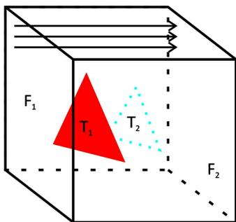
Fig. 3: Technique for determining internal block occlusion using an approach similar to Z-buffer. When verifying the visible set of Triangles for face  $F_1$ , the rays determine that triangle  $T_1$  hides triangle  $T_2$ .
