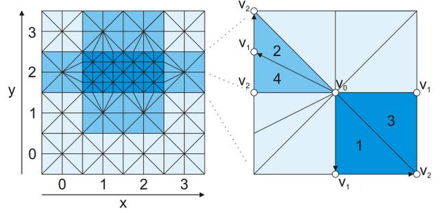
Fig. 2: 2D example for a triangulation grid  $J_1^a$  (left) and details of the block  $g = (3; 2)$ ,  $r = 0$  where it is shown two paths for tracing the block simplices.
