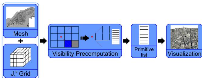
Fig. 4: Overview of the processing pipeline for visualization.
